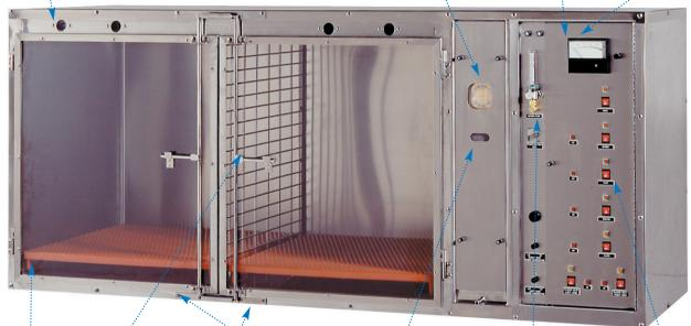
Plastisol-coated Cage Floors are included for patient comfort. Removable wire grill and clear acrylic panel (included) slide into rear channel to create two compartments. Built-in floor heaters provide even, steady heat to help maintain the patient's body temperature. Monitoring window lets you visually check when the carbondioxide filter needs to be changed. Oxygen flowmeter regulates the flow of oxygen delivery.
