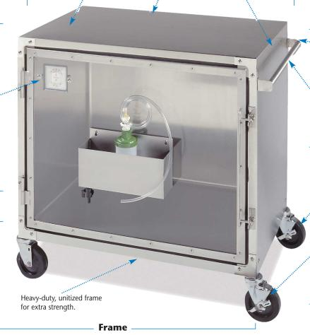
Thermometer/hygrometer monitors temperature and humidity. .
