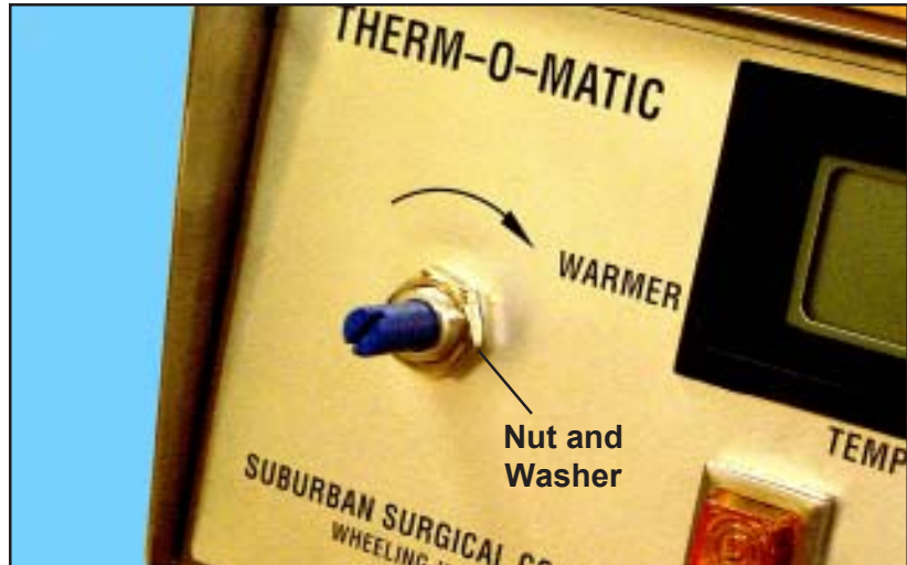
Figure 20. Heat Controller Nut and Washer
