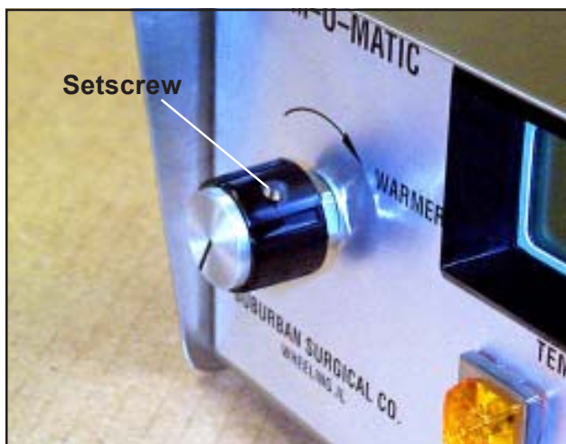
Figure 18. Temperature Control Knob Set-screw
