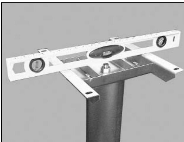
Figure 2. Checking Level Right-to-Left
