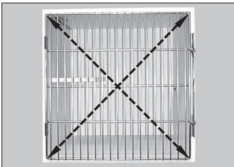
Figure 54. Measuring the Door for Deformation
