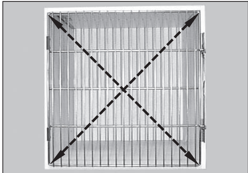
Figure 61. Measuring the Cage Door for Deformation
