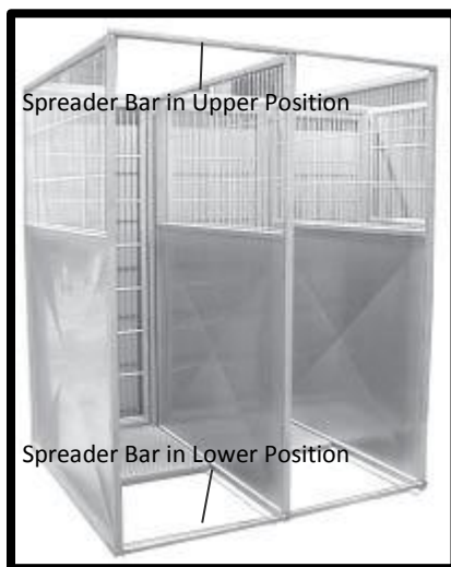
Figure 33: Back Spreader Bars on Pens
