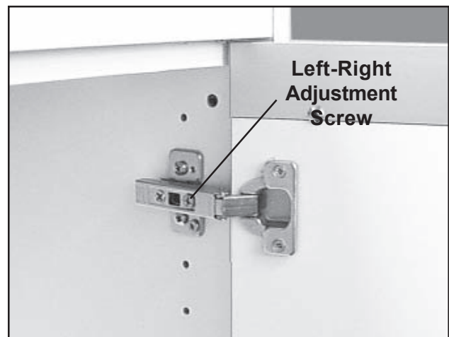
Figure 10. Door Left-Right Adjustment Screw
