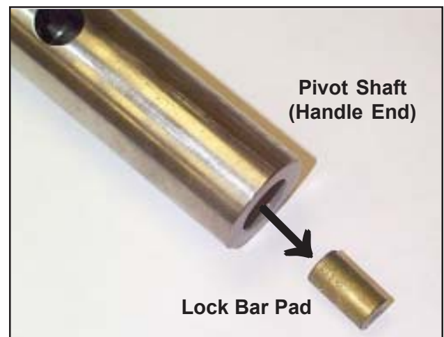
Figure 33. Removing the Lock Bar Pad from the Pivot Shaft
