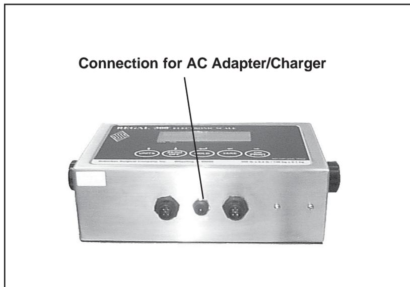
**Figure 34. Removing the AC Adapter/Charger Wire**
