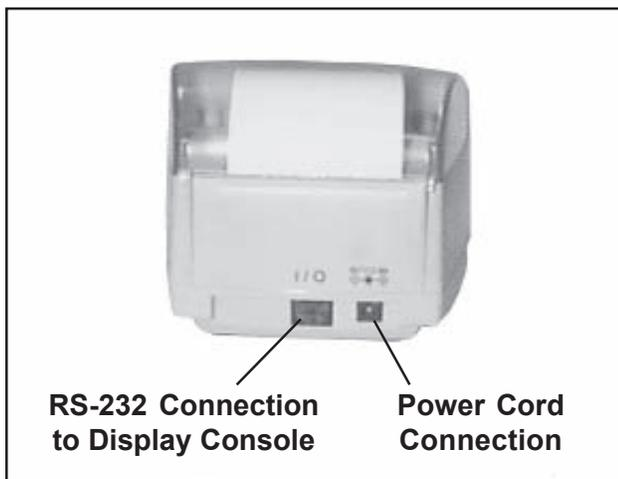
Figure 16. Printer Cable Connections
