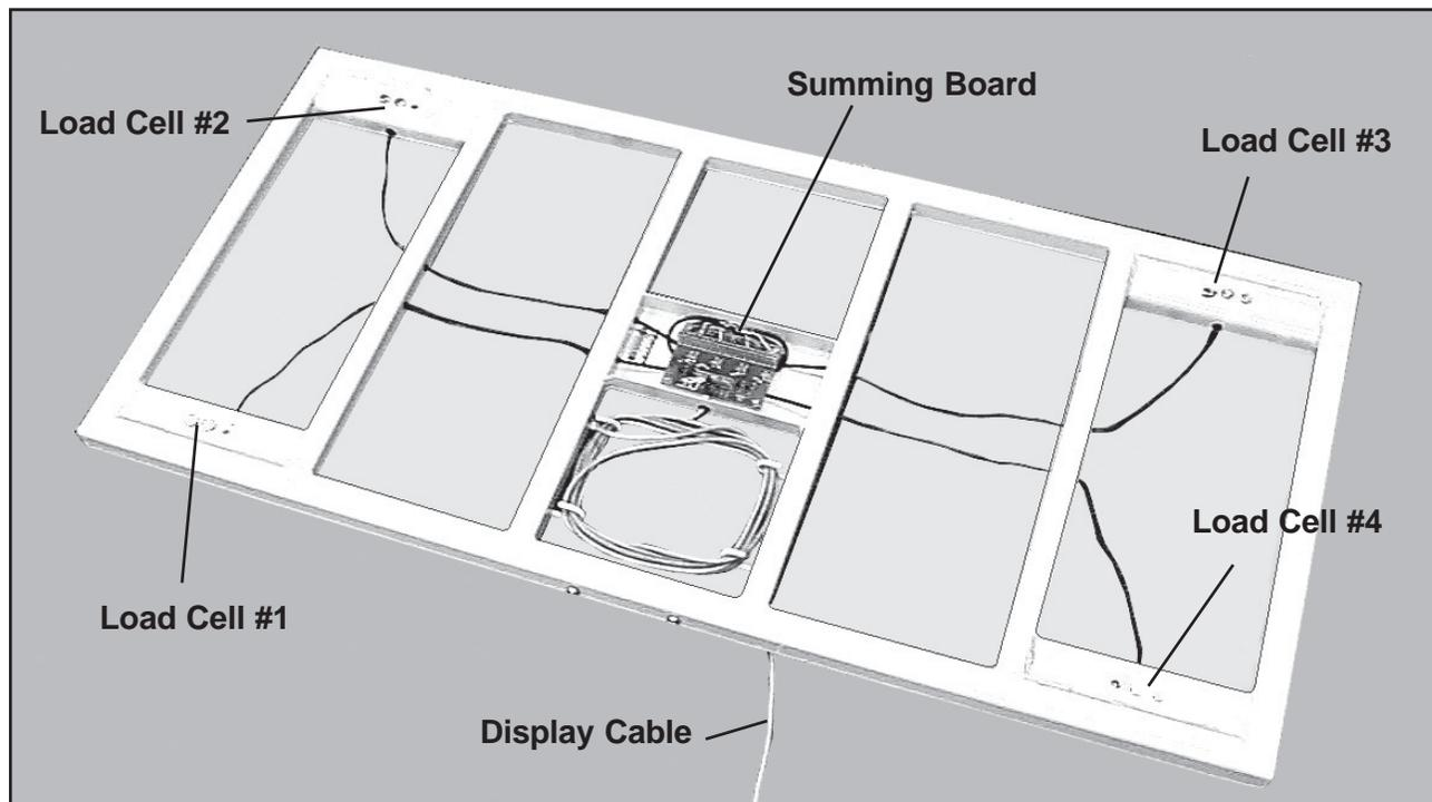
Figure 47. Overall View of Platform Frame, Load Cells, & Summing Board
