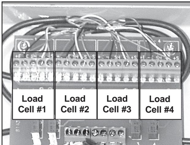
**Figure 50. Load Cell Wiring Groups**
