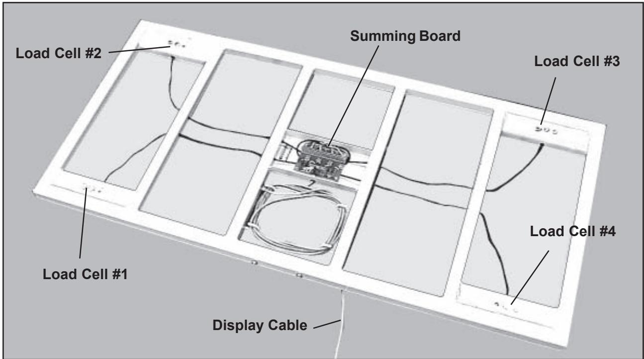
Figure 55. Overall View of Platform Frame, Load Cells, and Summing Board
