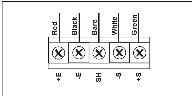
**Figure 58. Load Cell Wire Connections to Terminal Block (same for all 4 Load Cells)**
