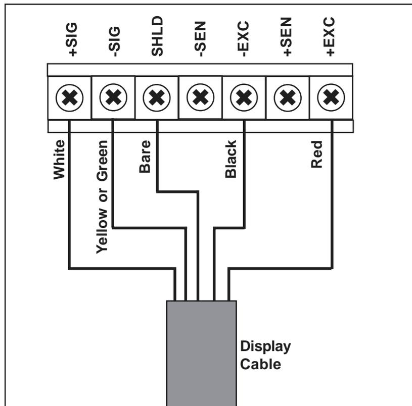
**Figure 54. Display Cable Wire Connections to Summing Board Terminal Block**
