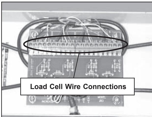
Figure 56. Summing Board - Load Cell Wire Connections
