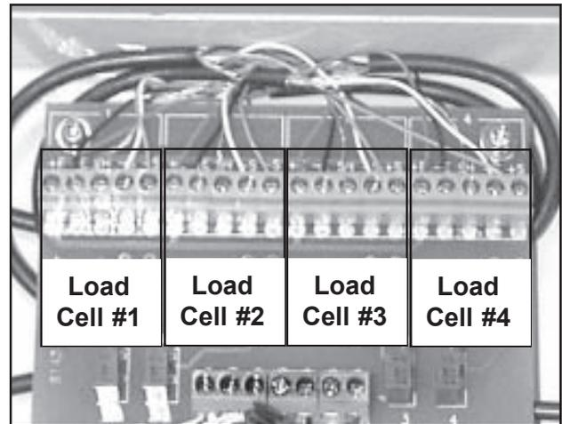
Figure 57. Load Cell Wiring Groups
