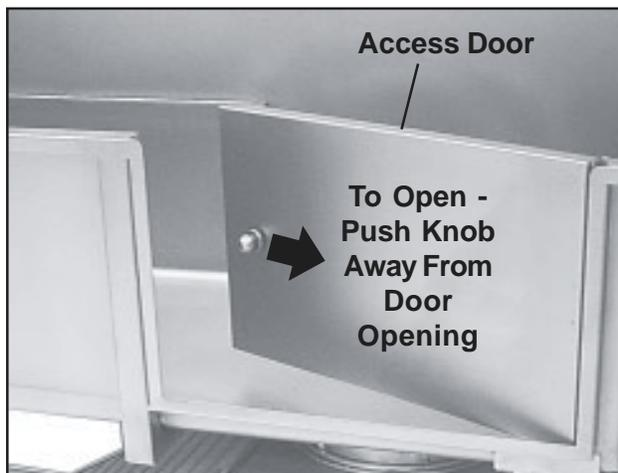
Figure 2. Opening & Closing the Access Door
